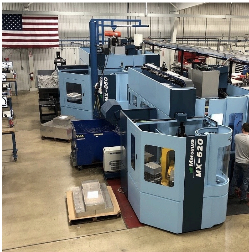
Figure 3. Matsuura MX-520 and MX-860 machining centers on a defense production floor.
